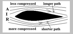
That is, the air above the wing just moves up a little, getting compressed, and the air below moves down (also getting compressed), so that the wing can slide though. As soon as the wing is past, the air expands back and returns to where it was before.
