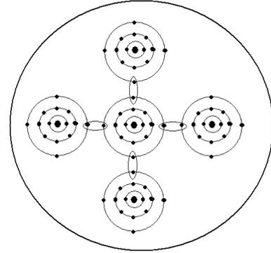
Now, if the crystal has a slight impurity of phosphorus, which has five outer shell electrons, the occasional phosphorus atom can stand in for silicon in the lattice, but this 'extra' electron is left not securely bound, and 'free' to move from atom to atom. The result is to make the crystal like a conductor, a semiconductor.
