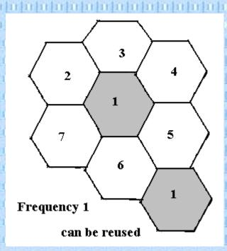
Cell phones satisfy the mobility need by being short-range radio sets. To provide a separate frequency to each phone, the cellular method 'reuses frequencies' by dividing the city into a series of hexagonal 'cells', as shown in the picture
