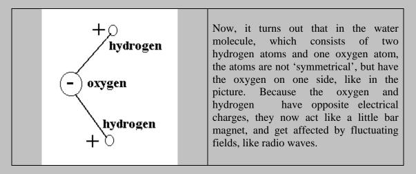
Normal radio waves are too slow to affect them in a major way, but microwaves are near the natural rotational frequency of water molecules and they set them spinning at tremendous speeds. This is what happens with the molecules of water in the liquid state, where the molecules are 'free' to move.
