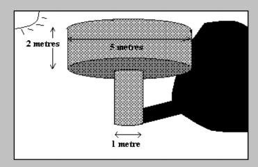
An example can be a water tank supported by a column, like in the picture. If the dimensions are doubled, then the diameter of the column goes from 1 metre to 2 metres. As the strength of the column depends on the cross-section area, the strength increases by a factor of 2x2=4.
