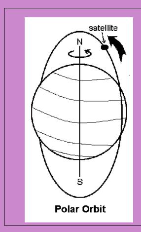
In the first kind, the satellite orbits in a north-south direction, or in a plane that contains the axis of the earth's rotation, like in the first picture. While the satellite goes around, north-south, the earth rotates, west-east and the satellite must find itself continuously passing over a different places on the earth.
