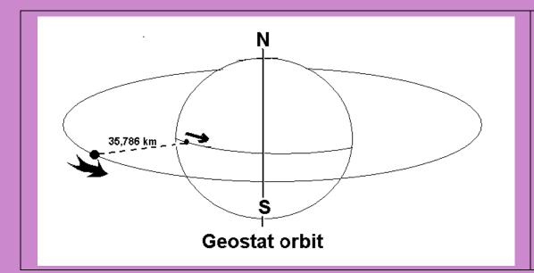
The satellite first launched so that it is nearly 'geostationary' and then allowed to drift till it is over the part of the earth where it is required. At this spot its speed is adjusted so that it becomes truly 'fixed' and can perform its function
