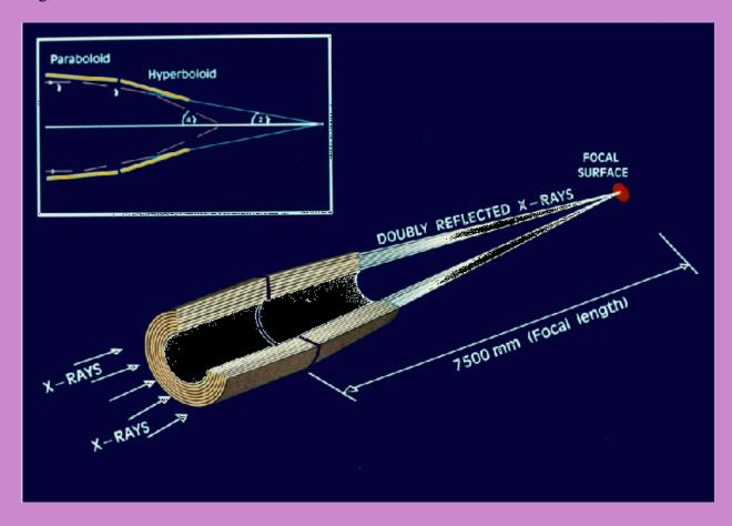
The X-ray Multi Mirror telescope, launched in 1999, contains three identical X-ray mirror assemblies with an outer diameter of 70 centimeters each. With a total of 174 mirror shells, a length of almost 10 meters, a diameter of four meters and a total mass of nearly four tons, this new telescope has relayed some breathtaking pictures of cosmic events.
