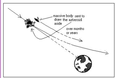
It has been worked out that a 20 tonne craft could safely deflect a 200 metre-wide asteroid in about a year. Given the ample warning that we would have about large asteroids, it is feasible that the craft be launched and put in position well in time.
