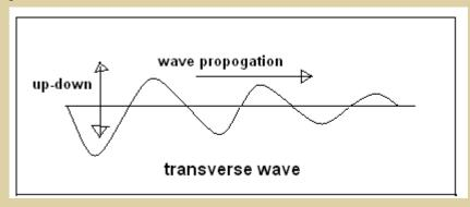
The speed of transverse waves depends on the properties of density, viscosity and surface tension of the medium, and in the sea, is a few kilometers an hour. But longitudinal waves depend on the elastic properties of the material – how fast it rebounds when compressed. And as water is practically incompressible, longitudinal waves in water travel at several hundreds of kilometers an hour!
