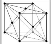
Now, if just an occasional silicon atom is replaced with an atom of a different element, which has either 5 or 3 electrons in the outermost shell, then that atom can also be in the hand-holding lattice, except that each such atom would have one electron too many or be one electron short. Treating silicon like this is called *doping*. This extra electron, or the *hole*, where there is one
