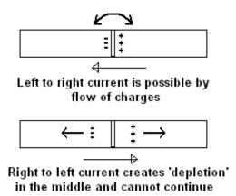
The combination of a photovoltaic material and such a semiconductor, which will carry away the electrons knocked out by light energy, but not allow the electrons to go back the same way, then drives the electrons round in a 'circuit' - thus creating and electric current.
