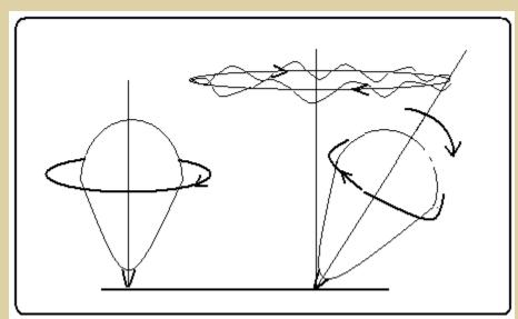
As shown in the picture, if the top begins to tilt to one side, which is to move downwards, this motion throws up a force that pushes the tilting axis of rotation in a horizontal way, to rotate about the vertical itself! This rotation is also a kind of 'spin' and this spin, in turn, generates a force to push the top upright again, and the tilt reduces. The reduced tilt reduces the horizontal motion and this again starts the vertical drop. Which increases the horizontal motion and so on.
