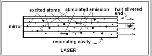
It was suggested in 2003 that a similar process could be used to amplify the plasmons within, or on the surface, of a metal, to help communicate with an external medium. The laser process is so named as an acro\nym for Light Amplification by Stimulated Emission of Radiation (LASER). The same thing for Surface Plasmons would then become a SPASER.
