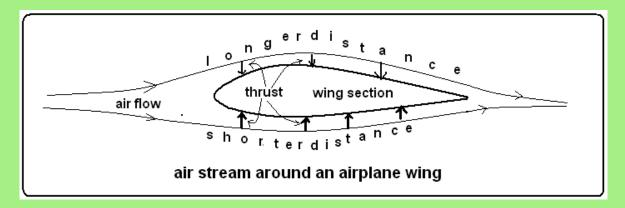
The theory is exact and simple so long as we are talking about air that moves *smoothly* around the wing. If the wing were to move very fast through the air, the relative movement would not be smooth, but would become turbulent, with whorls, eddies and uneven pressure distribution, which complicates things. The sensitive control that living things, like birds and insects, can exercise over flight seems to come from control of these complex features of fluid dynamics.
