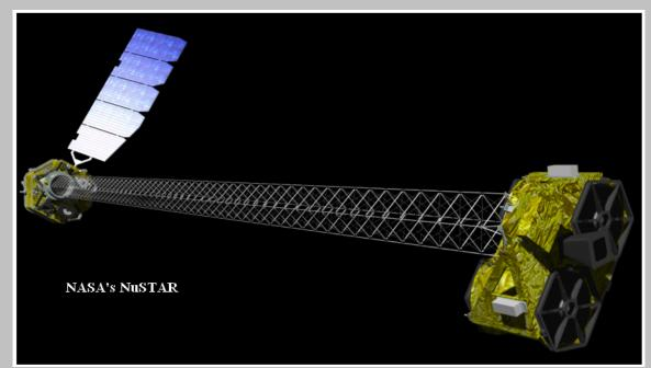
The NuSTAR optics enables detection of X Rays of about ten times the energy, or about ten times shorter wavelength than the SMM-Newton, which is a very great advance in sensitivity.
