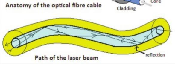
which guides laser beams along its length. The laser beams traverse the fibre by reflecting off its sides at a glancing angle. Rapid, electronic offand-on switching of the beam allows digital data to be transmitted with great speed and accuracy. By using different glancing angles, many beams of light can be sent at the same time and a cable with a bundle of fibres can carry huge data.
