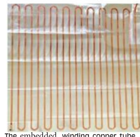
The embedded, winding copper tube that carries water.
