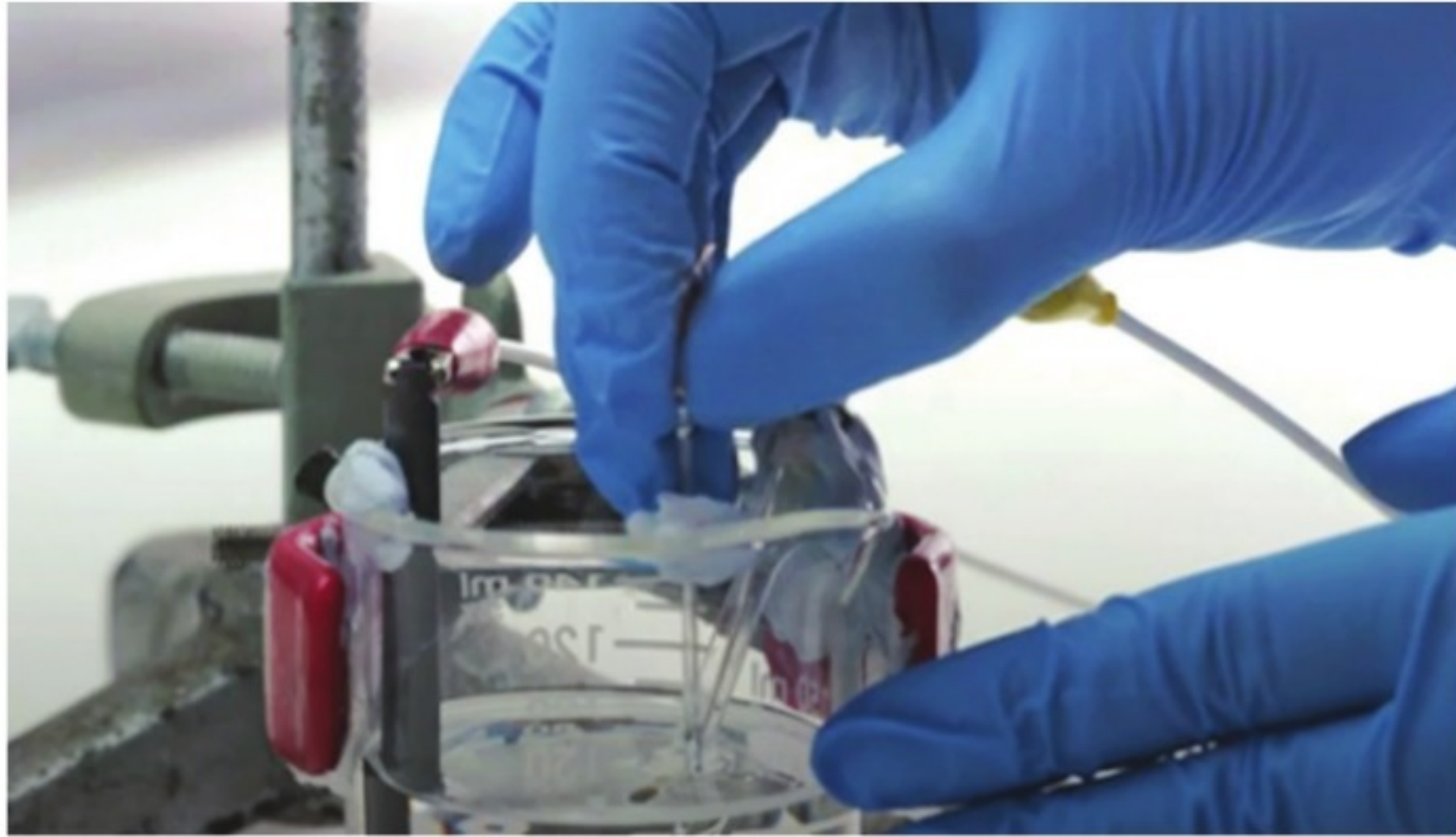
Electricity through CO 2 using liquid gallium as electrode, with cerium oxide nanoparticles in suspension.
