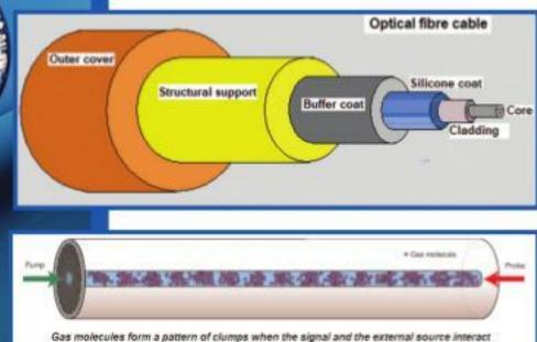
"pump" and the "probe") is to get the gas molecules to form periodic lumps.
