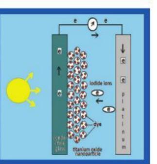
for use in conjunction with the current one, to enable the device to react to more parts of the spectrum of the incident light. The additive also prevents electrons that are emitted from being captured by neighbouring dye molecules before they move through the circuit. The result is greater production of electrons, a voltage of 1.24V or power conversion efficiency of 13.5 per cent. The DSSC is hence suitable for use in cloudy conditions or to power indoor devices, a press release says.
