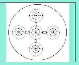
Now, if the crystal has a slight impurity of phosphorus, which has five outer shell electrons, the occasional phosphourus atom can stand in for silicon in the lattice, but this 'extra' electron is left not securely bound, and 'free' to move from atom to atom. The result is to make the crystal like a conductor, a semiconductor.
