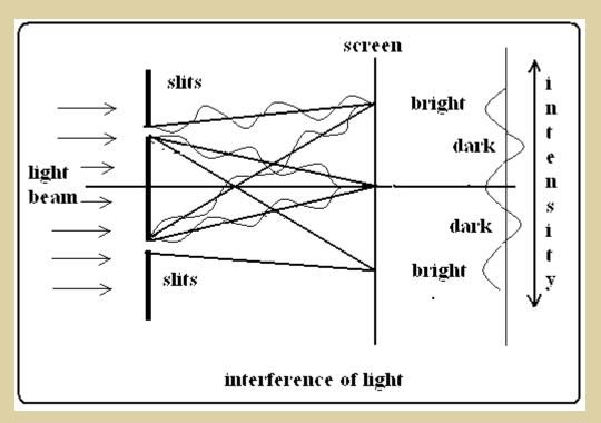
This pattern of bands can be made very much more intense and sharp by using a large number of parallel slits. An arrangement like this, which is made by ruling lines on a glass sheet, is called a *grating*. As the wavelength of light is extremely small, of the order of millionths of a meter, the lines are also very close together, like thousands in a centimetre.
