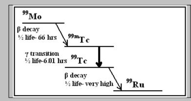
The <sup>99</sup>Mo is itself produced in nuclear reactors, when enriched <sup>235</sup>U, or a radioactive form of uranium, in a concentrated form, is bombarded with neutrons. The decay of the <sup>235</sup>U, gives off two neutrons of its own, which can induce more decays, and so on and this is the principle of the nuclear chain reaction of nuclear power plants and atom bombs. <sup>99</sup>Mo is thus extracted
