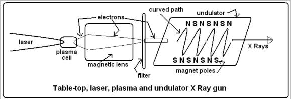
The electron beam is then passed through an 'undulator', a series of opposite pole magnets, just 30 cm long with magnets 5 mm apart, which twist the high speed electron beam into a rapidly curving path. The result is X Rays of the ultra short wavelengths of synchrotrons and free energy lasers, but through a table-top arrangement!
