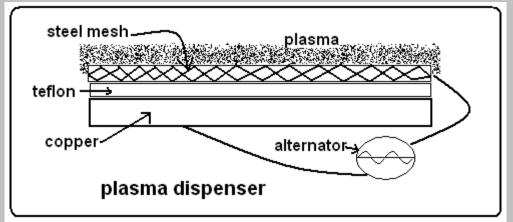
Plasma is created within the mesh, it barely warms up more than 5 degrees C, can cover comfortably the area of a pair of hands and clears bacteria down to nearly a millionth of its population in less than 10 seconds. The device generates UV radiation or toxic gases within permitted limits and is within safe limits of electrical current and voltage.
